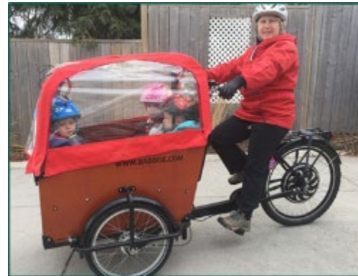
Reverse tricycle design with enclosed cargo box in the front
