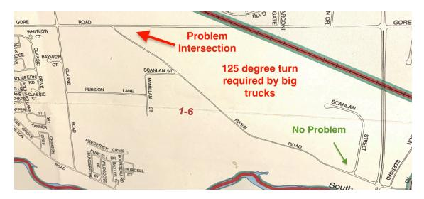
To navigate the exiting turn eastbound, trucks have to move into the oncoming River Rd lane and turn into the oncoming Gore Rd lane. Sometimes the turn is cut too tightly and they drive over and damage the curb which can be seen in the photo below.
