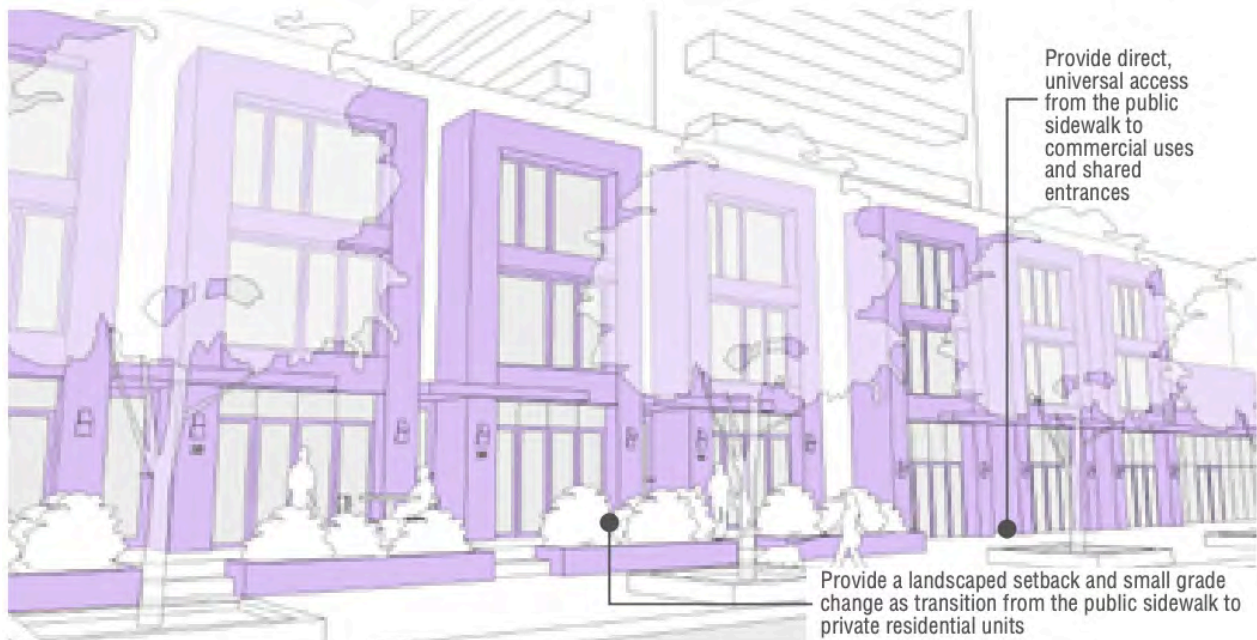
Figure 1: Treatment of the transition space between the public sidewalk and building interior reflects the differing needs for access and privacy between residential and commercial frontages.
