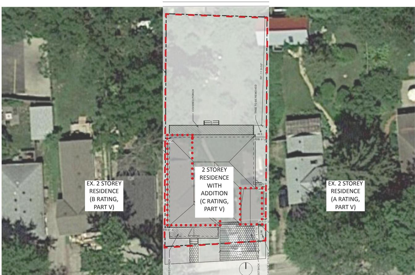
Image 15: Site Plan of Proposed Addition/Renovation, 18 Byron Ave E. Green shaded area indicates new footprint of proposed residence (not include front and rear porches). Red dotted lines indicate location of original house and garage to be incorporated within the proposed addition and connected to create one larger residence. Diagram prepared by a+LiNK architecture inc (2021).
