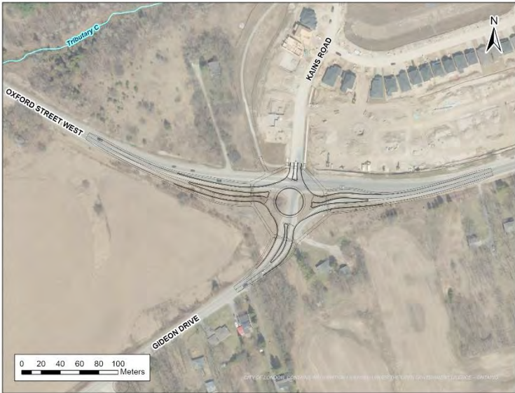
Figure 7.3 – Alternative Solution 3 – Single-Lane Roundabout
