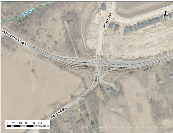
Figure 7.4 – Alternative Solution 4 – Multi-Lane Roundabout
