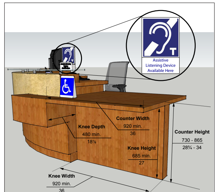
Figure 110: Dimensions of Accessible Service Counter
