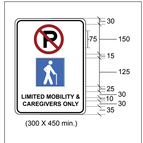
Figure 27c: Type C Vertical Signage - Detailed Dimensions
