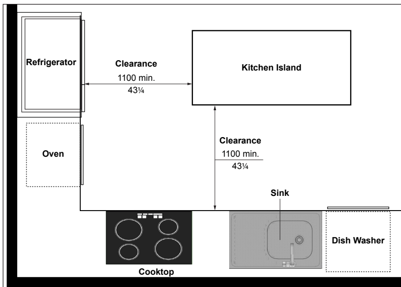
Figure 94: L-Shaped Kitchen - Plan View
