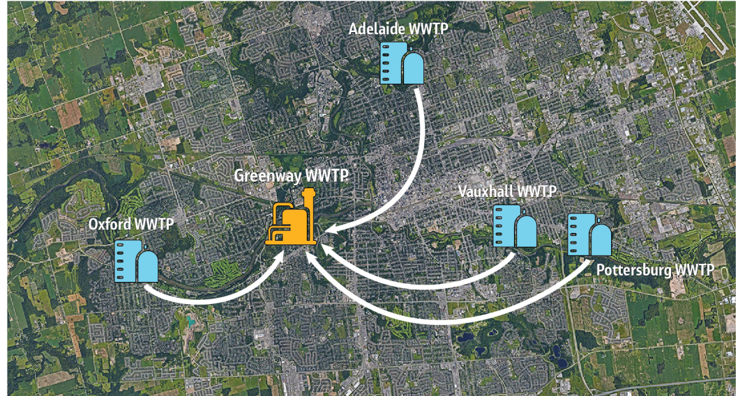
Solids Trucking to Greenway WWTP
