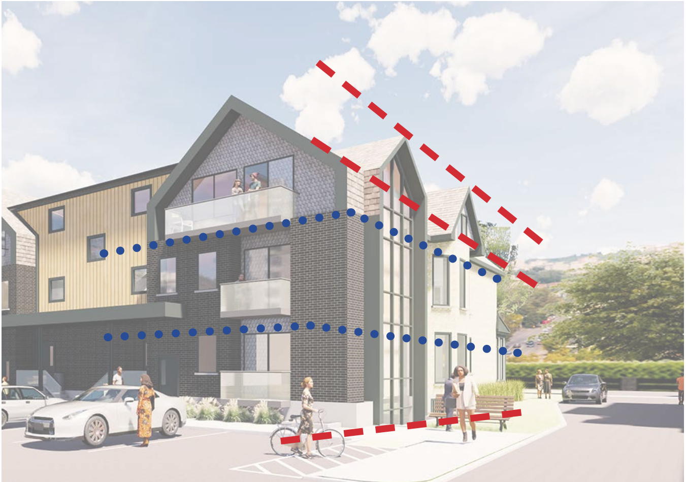
Image 32: Massing Diagram- Southwest Elevation. Red dashes indicate aligning gable pitches, heights, setbacks, and building facades of the addition and the original buildings. The blue dots highlight the fenestration and separation of windows on each level, carried onto the addition from the original building. Note the two and a half storey glazed wall that creates a pause between the new and the existing at the addition on the south elevation, but also provides a sense of transparency while reflecting the context of the adjacent surroundings. Newly integrated landscaping has improved the design of the laneway and the rear parking area provide improved access to the property and the building, vibrancy and enhancement to the property. Diagram prepared by a+LiNK architecture inc., 2020.
