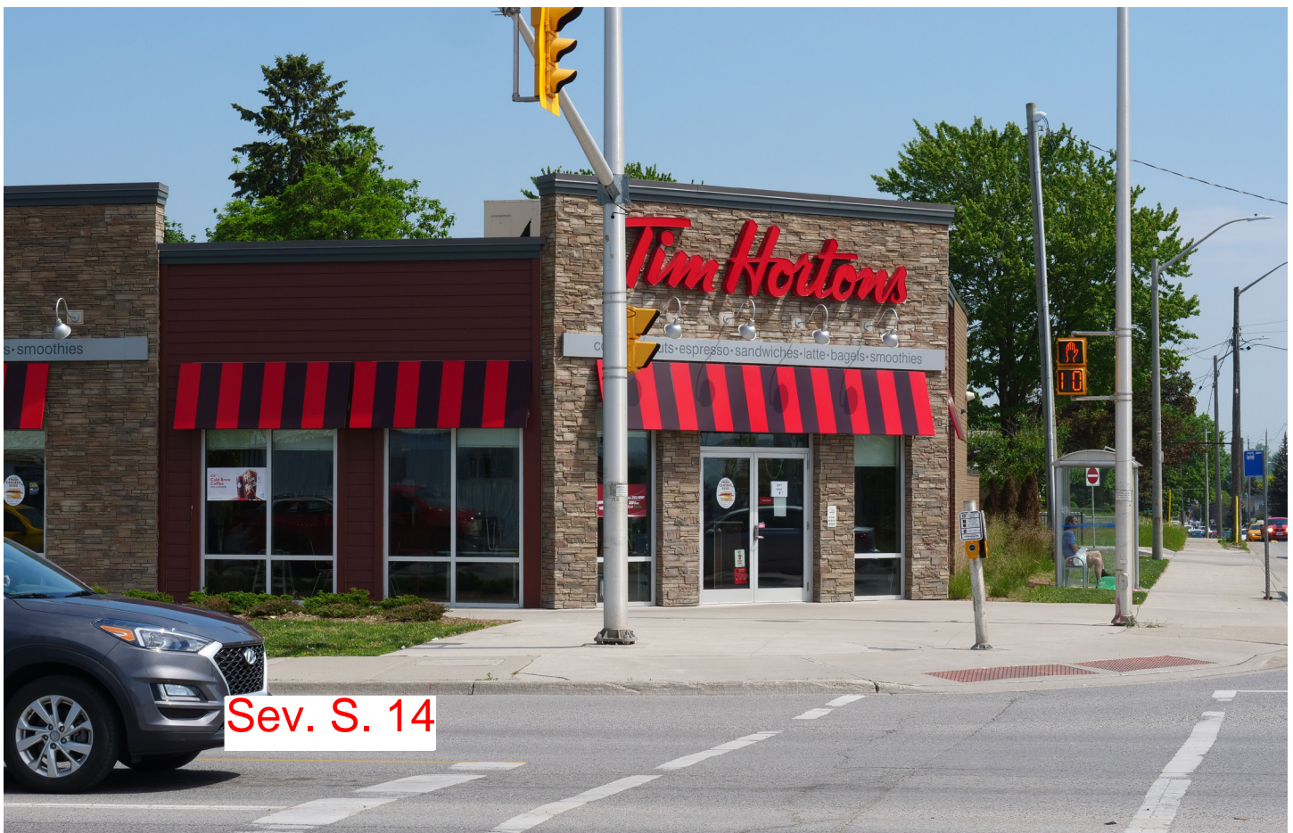
This cafe in London features the primary entrance oriented towards the street which provides direct access for pedestrians without having to walk through parking areas or drive-through lanes.
