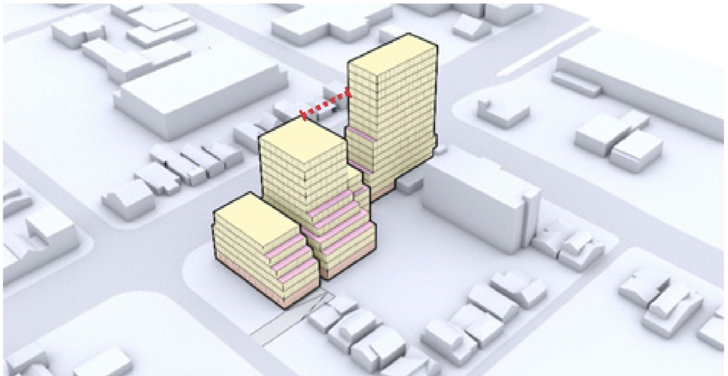
This image shows an example of high-density development. The red dotted line highlights the tower separation.
