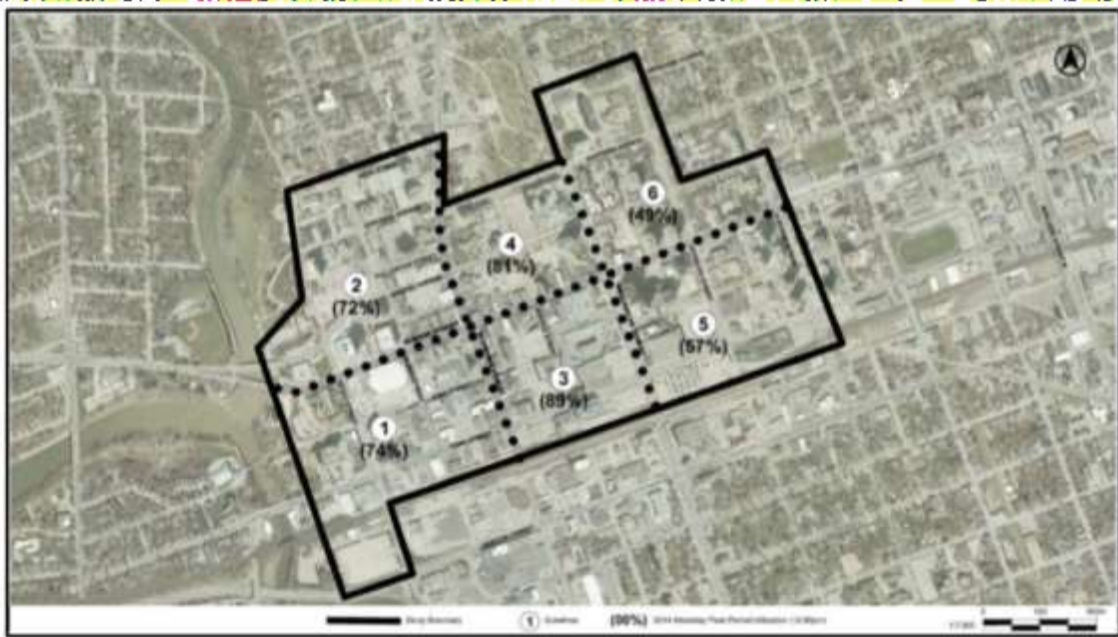
Figure 2: Parking utilization by sub-area, based on 2014 data.
