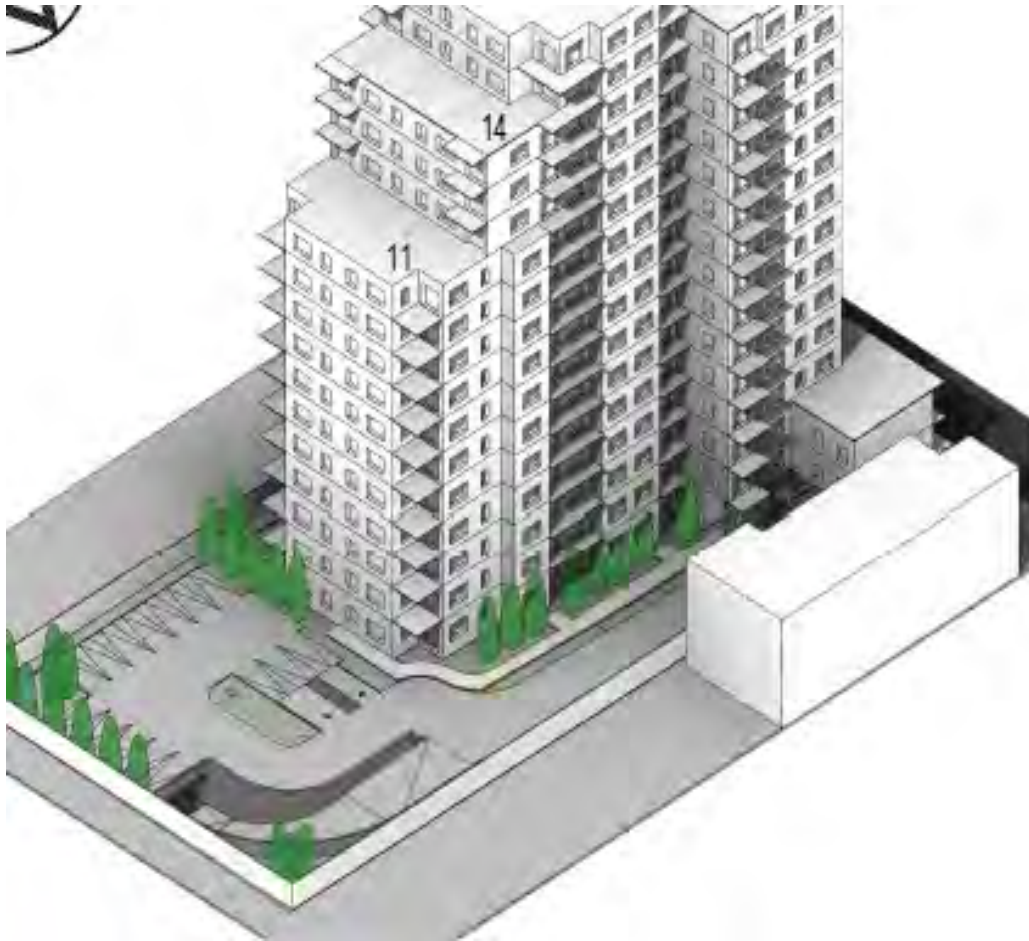
Figure 29 – (Above) Massing model of proposed development looking westward showing stepbacks on third and 15 th floor; (Below) Massing model from the rear demonstrating stepbacks on the 11 th , 14 th and 16 th levels (Source: Zedd Architecture, 2020)
