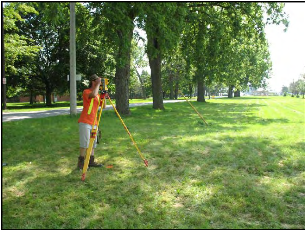
Image 11: Grid Survey with Total Station (looking southwest)
