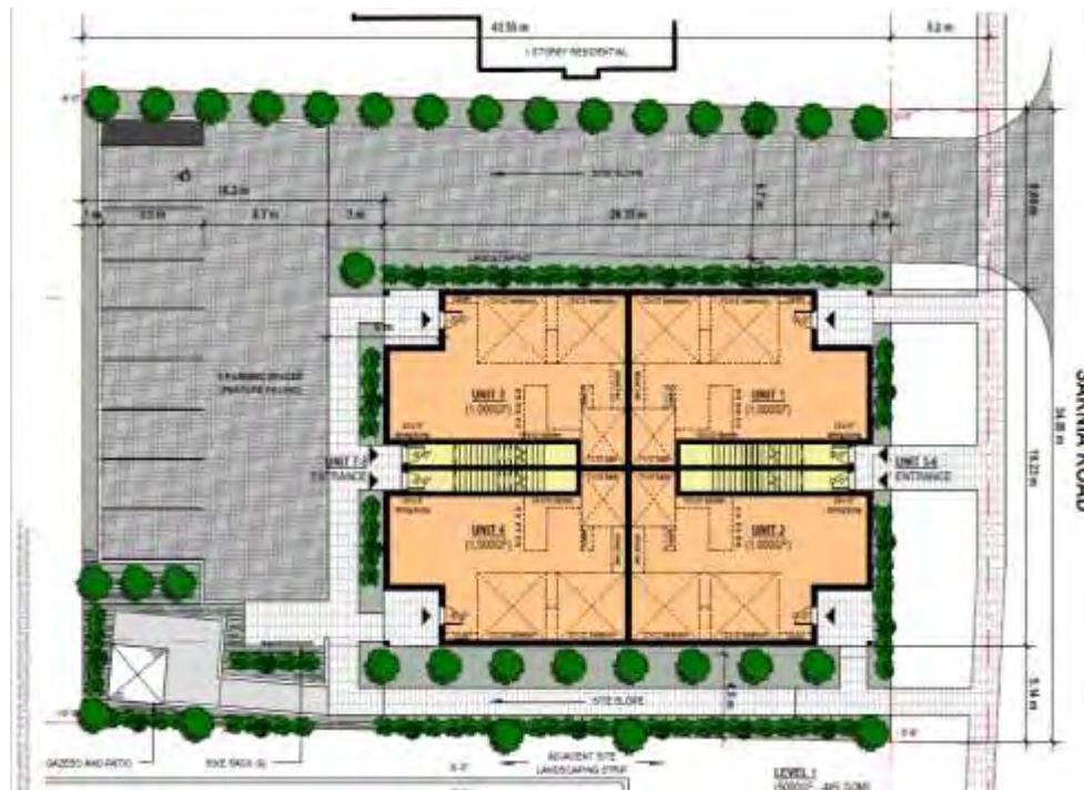
Figure 9: Site Plan and Ground Floor of Proposed Development at 260 Sarnia Road (Source: Zedd Architecture, 2020)
