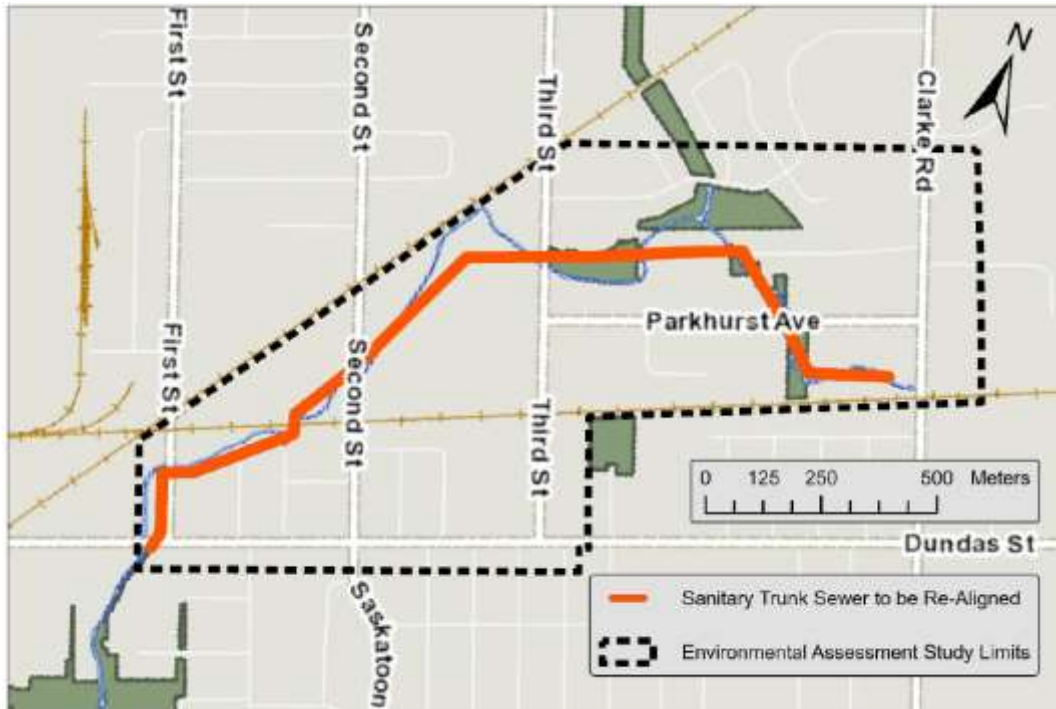
Figure 17: Study Area Pottersburg Creek Trunk Sanitary Sewer
