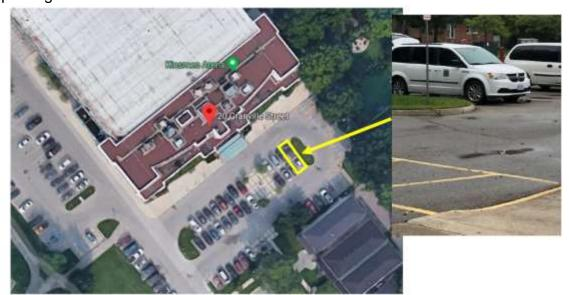
Electrical wires will run along from electrical room (southeast corner of the building) to the EV charger beside the island. A boring to the island will be applied to prevent any impact to the parking lot.
