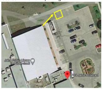
The electrical capacity has been confirmed for this location during the site assessment, and the wiring will be run from the electrical room to the North/East corner of the building. From there, it will be either bored or excavated to the north parking lot, as indicated with yellow square.
