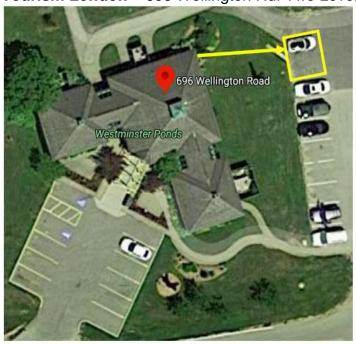
The electrical panel has space for two level 2 chargers and the designated EV parking spots are located behind the office. The electrical conduit can be excavated and buried in the lawn, and a concrete base is used for mounting the charger.
