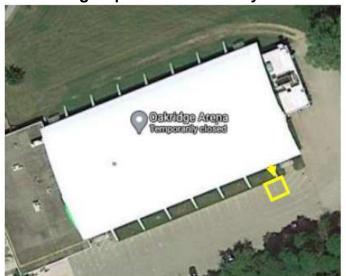
Two Level 2 EV Chargers located on the South/East corner of the building. The electrical can be run inside from the electrical room to the location of the chargers. We can use precast bases for mounting the EV Chargers.
