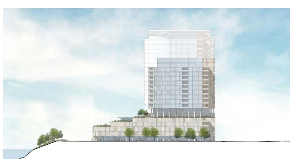
By aligning the towers and elongating them in a north-south orientation, the view obstruction from downtown is minimized, there's a greater feeling of openness and controlled solar gain, allowing ample daylight into the buildings which reduces energy consumption. This view is from west of the development.
