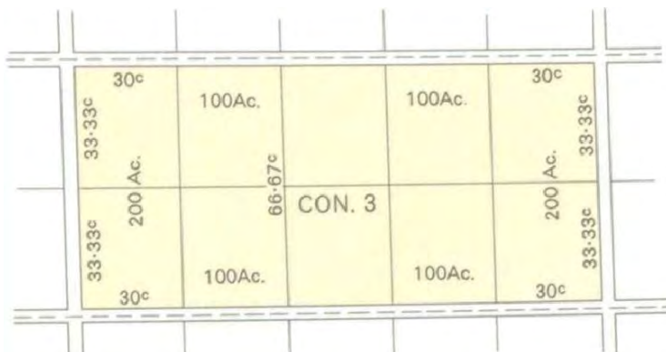
Plate 1: Double Front Survey System (Dean 1969)
