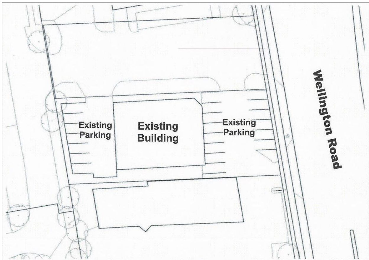
Figure 2 – Conceptual site plan submitted by the proponent illustrating the existing building and 21 parking spaces to be retained and used for the requested uses.
