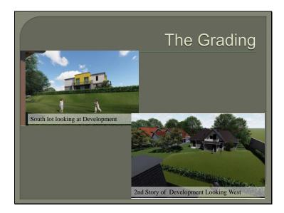
The first issue with the proposed development is the grading, or raised plateau that will be necessary to level out the topography of the lot. At the south end of the lot, the grading will be approximately 8 ½ feet in height, making the 2 ½ story stacked town house (Building #2) [click] appear more like a 3 ½ story which will in fact, tower over the surrounding houses, which are only 1 and 2 stories in height..
