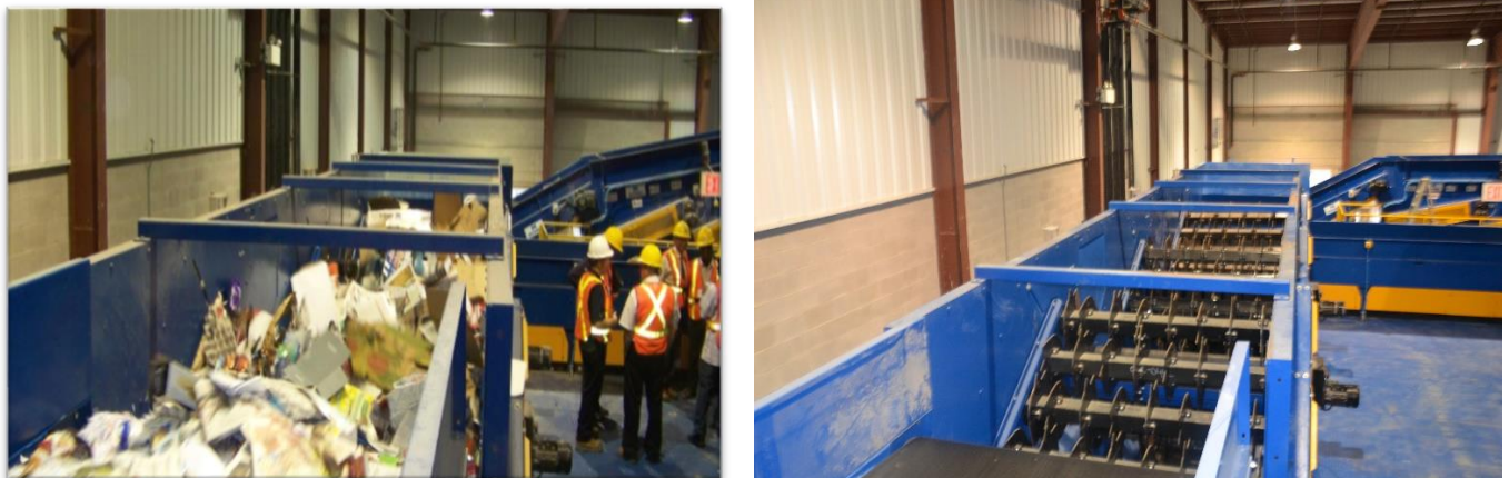
Figure 1: Paper products moving across the triple deck OCC sorter. Upgrades will be made to this piece of equipment
