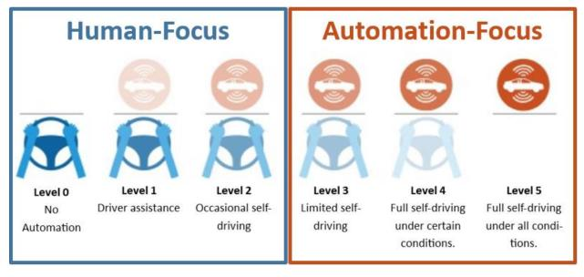
The key distinction is between SAE Levels 2 and 3, where SAE Level 3 begins to focus more on the automated systems monitoring the environment and performing the entire driving task.
