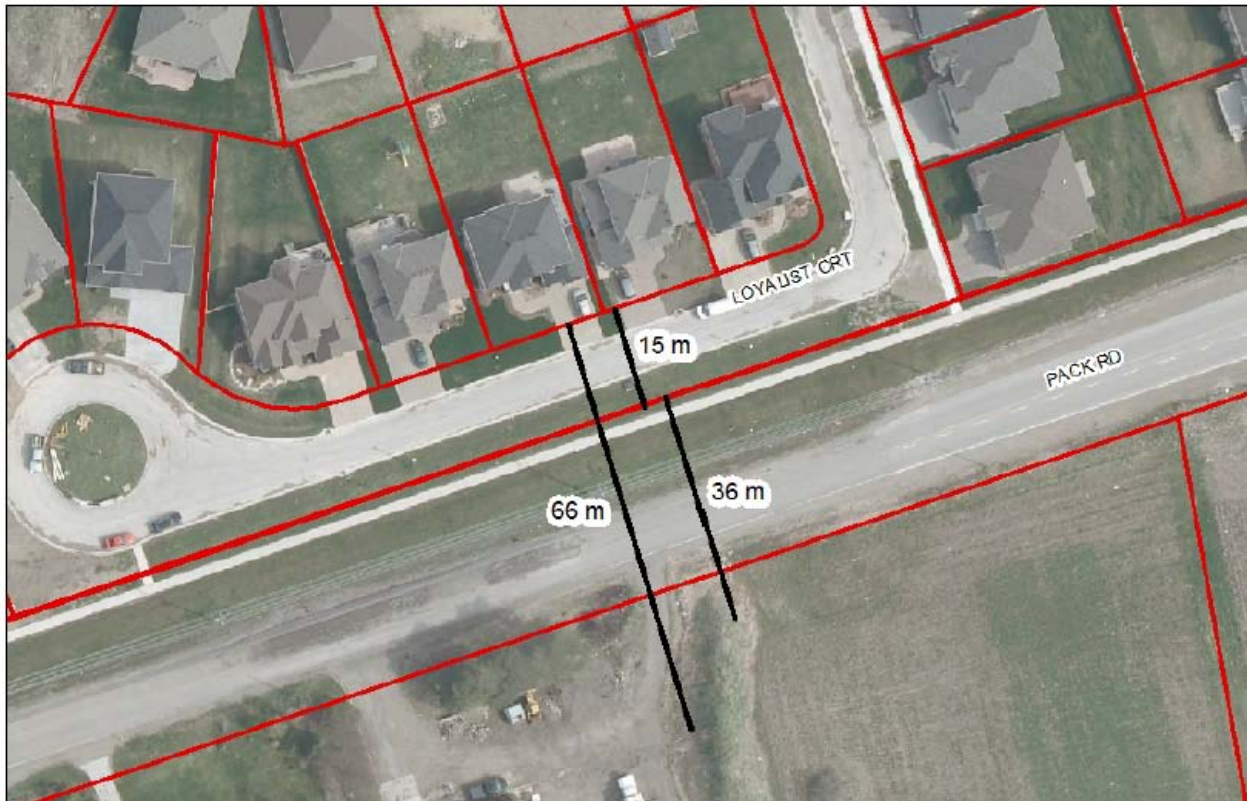
Figure 3 - Pack Rd: Illustration to show an example of a total 66 metre width along Pack Road, which includes a 36 metre right-of-way for Pack Road, plus the 15 metre wide window street for Loyalist Court and a second possible 15 metre wide window street on the south side of Pack Road.
