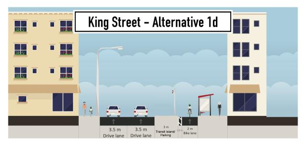
The most significant challenge for 1d, similar to 1c, is the high frequency of conflicts between transit passengers and cyclists. The bus stop does provide a refuge for passengers who are wanting to board the bus, where alternative 1c does not. Where there is no transit island, the parking lane is adjacent to the bike buffer. For this alternative, buses share the through lane adjacent to the transit island/parking lane and stop in the through lane during boarding and alighting.
