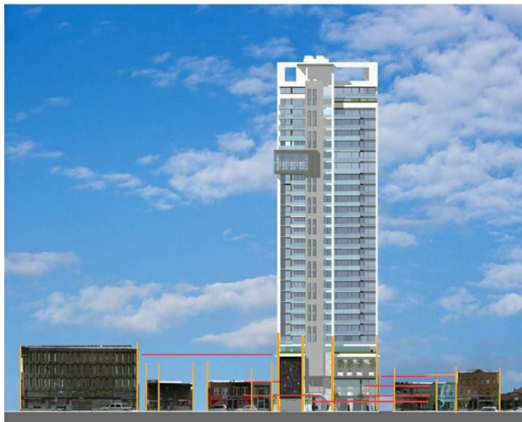
36. The coloured north elevation drawings showing a complex response to the existing cornice heights of adjacent buildings. On the King Street block.
