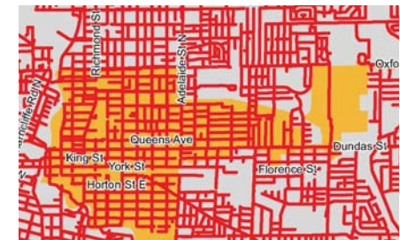
Sanitary Sewer System overlaid onto CASS area
