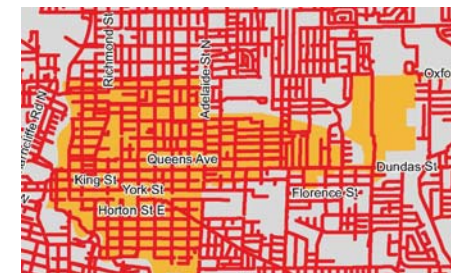
Sanitary Sewer System overlaid onto CASS area
