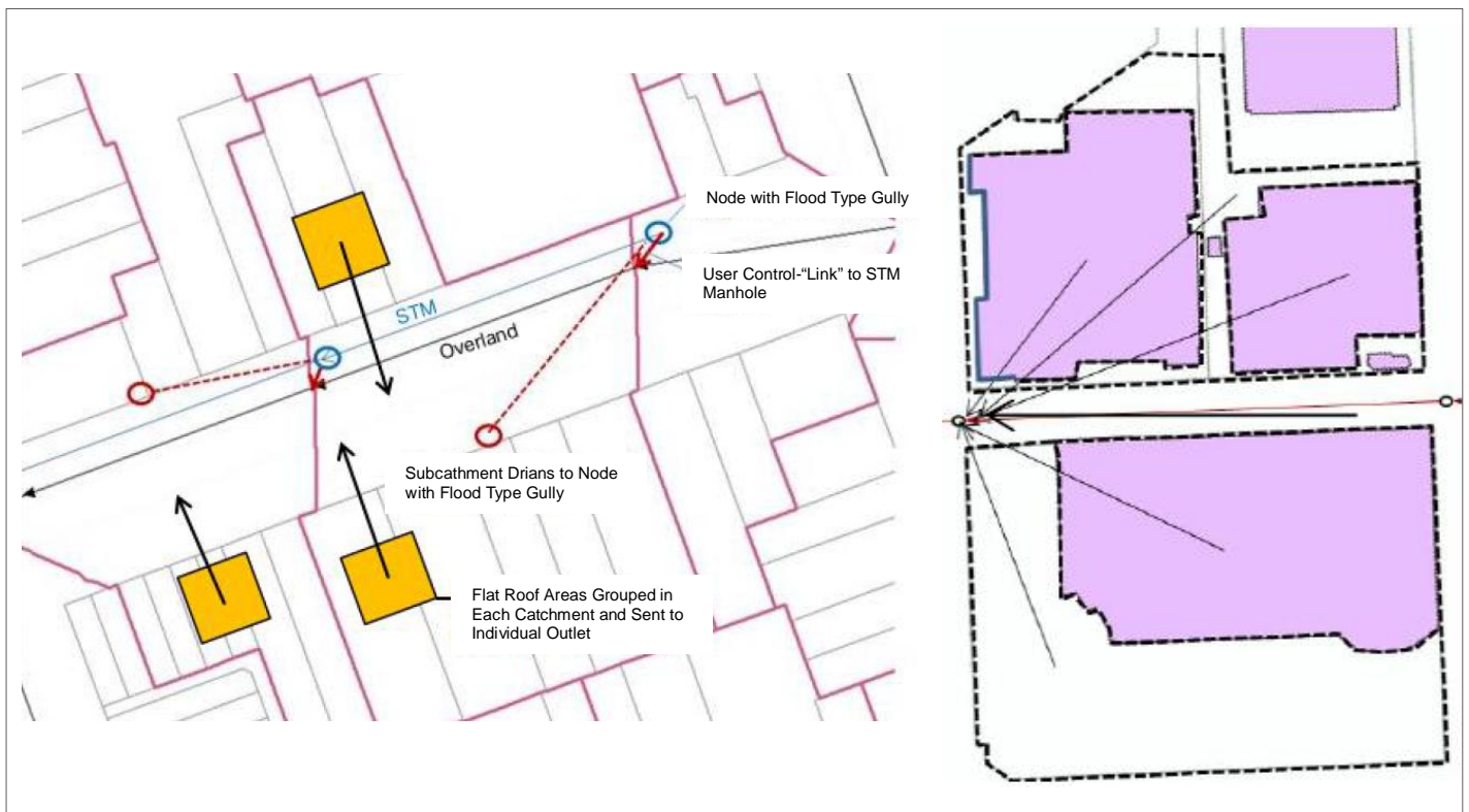
Figure 22: Schematic Representation of Storm Model Catchments
