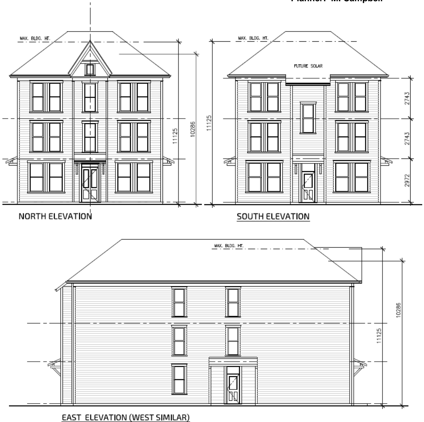
Figure 3: Proposed Building Elevations (467-469 Dufferin Avenue)
