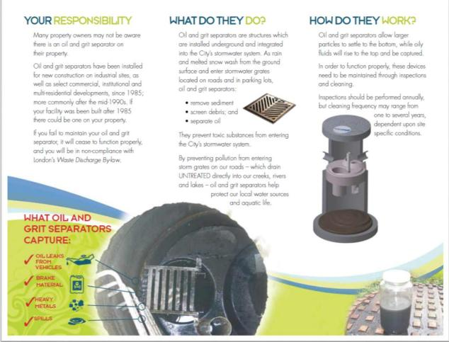
Figure B6: Stormwater Oil and Grit Separators
