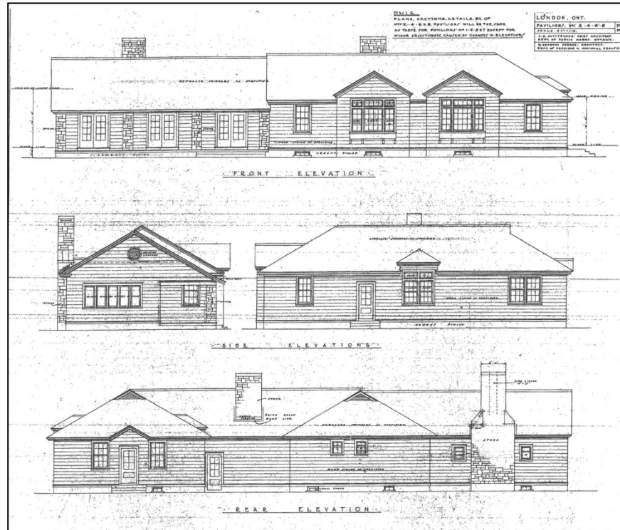
Figure 9: Elevations of cottage pavilions, originally clad in wooden clapboard. Source: Historica Research 2000.
