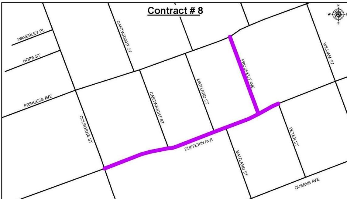
The construction program also includes replacement of lead water services, replacement of private drain connections (PDC), replacement of curb and gutter, new sidewalks and full asphalt road replacement for the full limits of construction. Improvements to the road geometry will be made on Dufferin at Cartwright to improve sight lines and assist pedestrian and safe vehicular travel through the corridor.
