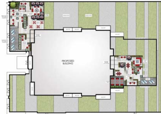
Roof Plan (showing green roofs and amenity areas on the 3rd floor podium and 11th floor roof)
