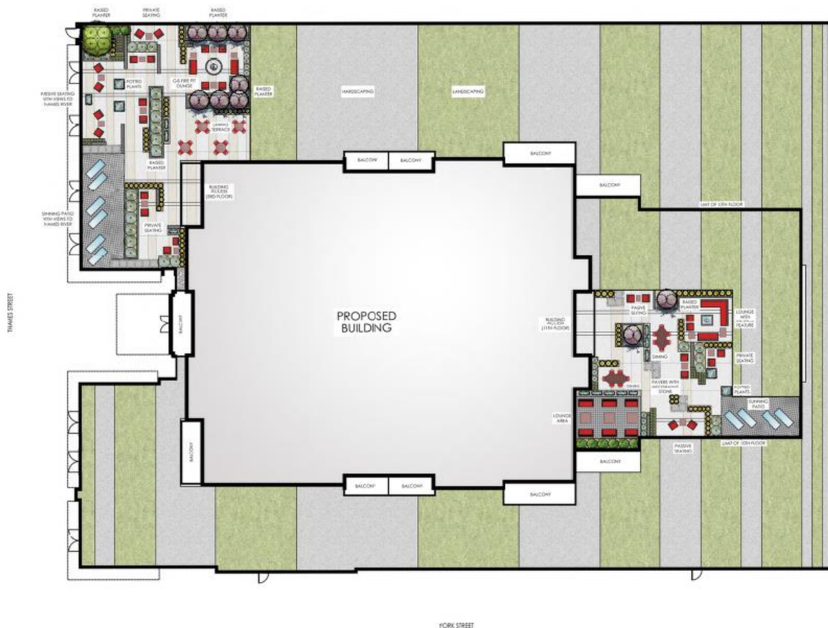
Below: Roof Plan (showing green roofs and amenity areas on the 3rd floor podium and 11th floor roof)
