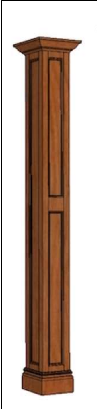
Image 3: Sample of recommended capital and base detailing for columns.
