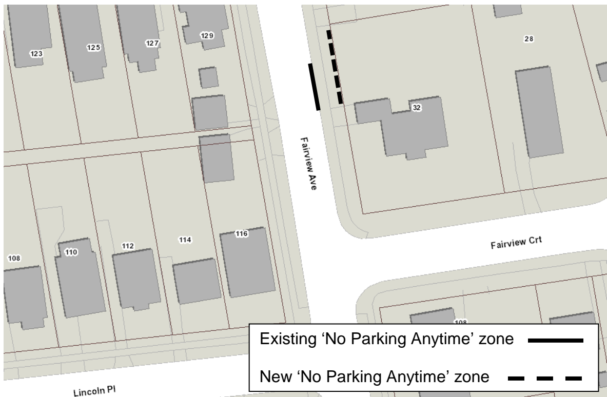
Figure 3: Fairview Avenue north of Fairview Court
