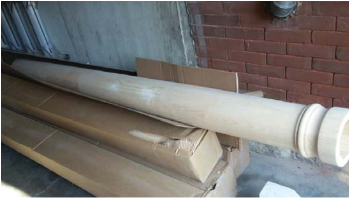
Standard wood, non-fluted, Tuscan capital available through column fabricators
