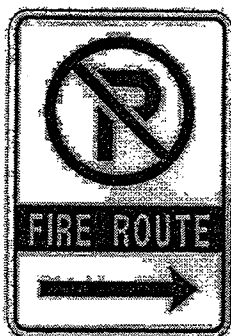
F.R. 2 Indicates direction of prohibited parking. Defines the end zones of a fire route.
