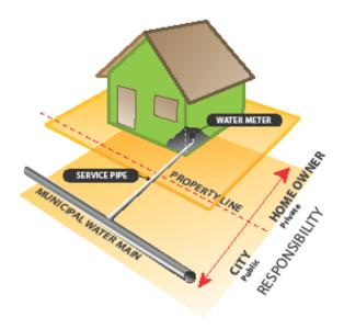
The water in London's distribution system has an extremely low level of lead, but the lead content in water can increase if the water travels through a lead water service pipe. The water service is the pipe that conveys water from the water main under the street to the
