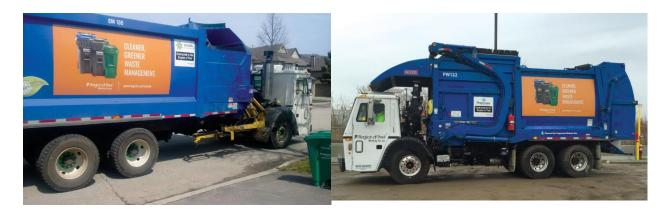
CNG garbage packers operate in the Region of Peel. One person, fully automated, side loader (packers) picks up carts at the curb (left photo). Right photo shows a CNG-powered front-end loader that collects bulk-lift containers.
