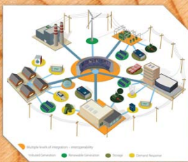
Smart Grid System Mesh-network where power flows from all the generating sources to the customers
