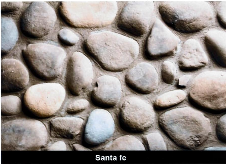
Image 6: Proposed field stone veneer material for porch skirting (submitted by applicant).
