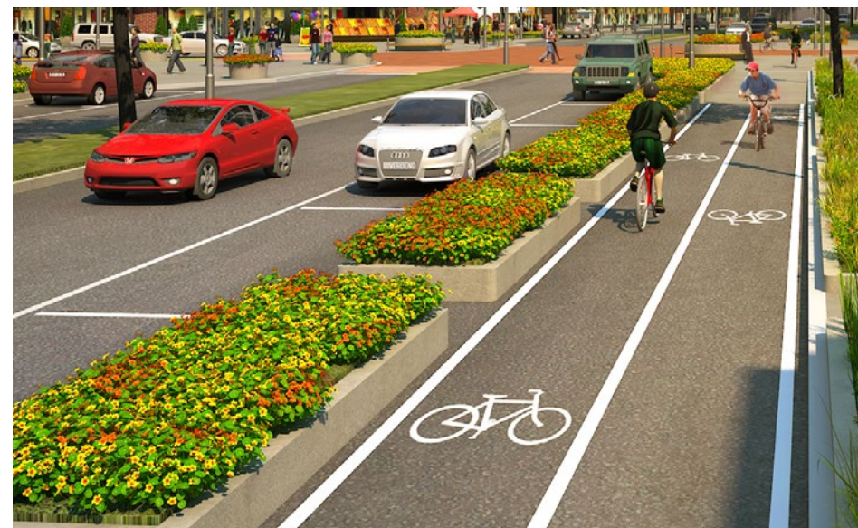
CONCEPT IMAGE OF BIKE LANES, PLANTER, AND PARALLEL PARKING ALONG STREET ONE. PLANTERS MAY BE RAISED OR FLUSH WITH THE ROAD SURFACE.
