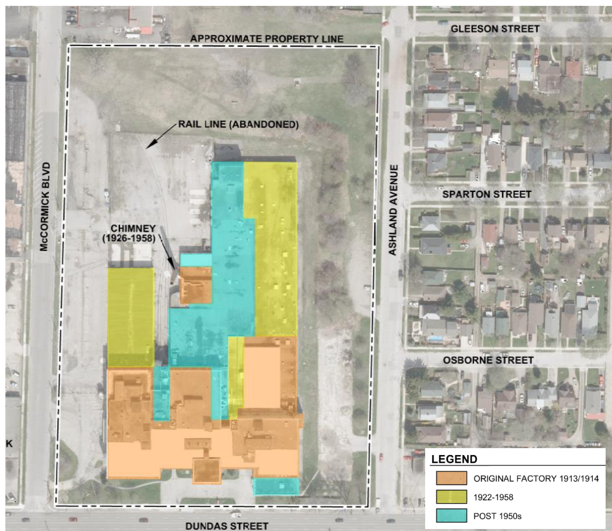
Figure 1 – Site Plan from Heritage Impact Statement showing dates of McCormick Factory Site Development. Please note that the property line shown is not correct but the purpose of the illustration is to show the building enlargements over time.
