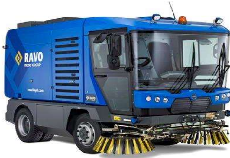
Figure 1, Ravo 5 iSeries – (Pure) Vacuum Street Sweeper
