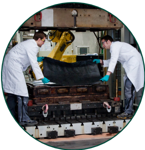
Dieffenbacher hydraulic high-speed press with a maximum press force of 25,000 kN (2,500 tons.)
