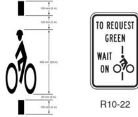
Figure 10-7. Example of Bicycle Detector Pavement Marking
