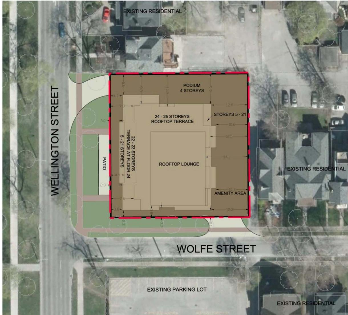
Figure 18: Site Roof Plan
