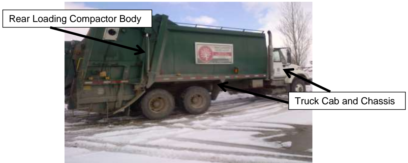
Figure 1 – 2005 International Cab and Chassis with Fanotech Rear Loading Compactor body
