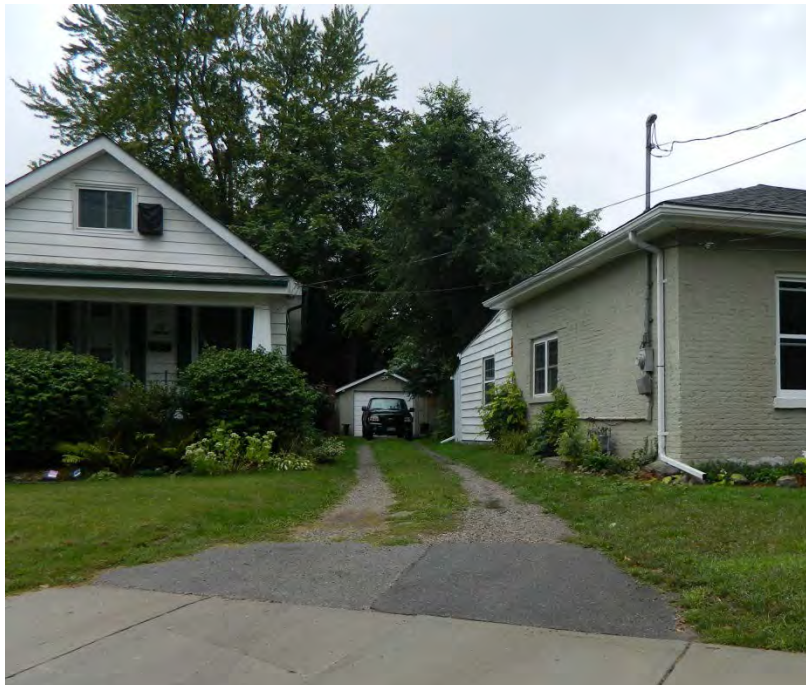
Figure 5: Use of two single track driveways minimizes large expanses of hard surfaces and softens the landscape between homes.
