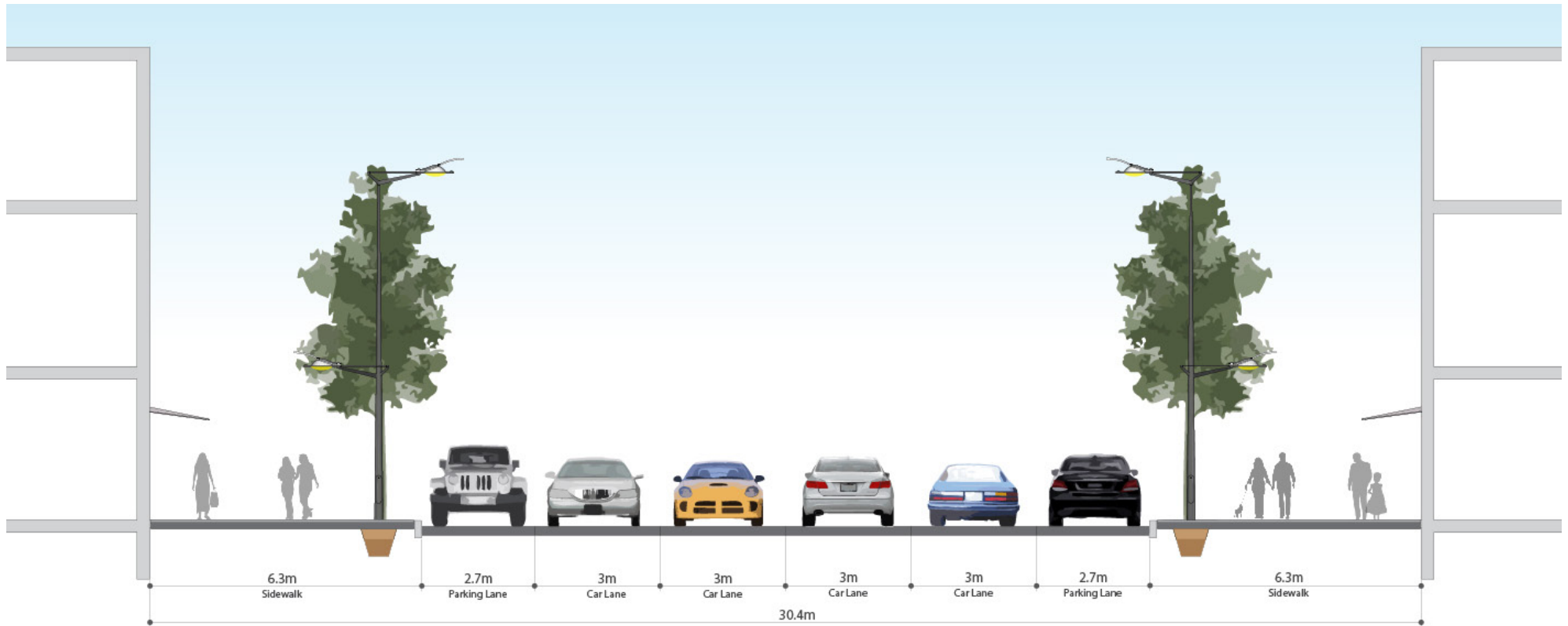
30M ROW - Mainstreet (non-site specific) Cross Section Detail
